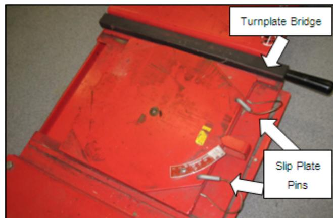
**Slip Plates** - The slip plates of a Hunter alignment rack are designed to move smoothly and freely to provide accurate measurements.
