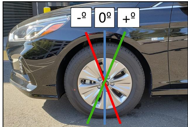
**Toe** The amount the tires point inwards or outwards when viewing the car from above.
