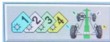
4. Continue to balance and tag all four assemblies. After all assemblies are completed, the screen will show display positioning and the effect on vehicle drift/pull or vibration. The purple horizontal arrow at the top of the screen displays overall pulling force and direction due to tire effects. The brown vertical arrows above each tire displays the RFV (road force variation) of each assembly.
