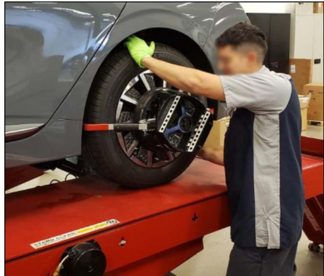
If equipped, ensure the pins are in the slip plates, and the turnplate bridge is oriented so that the bridge is level/flush with the rolling surface to minimize the vehicle's suspension movement.
