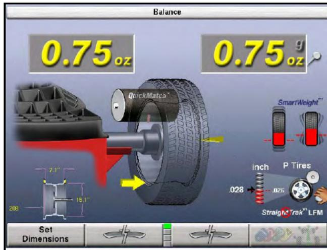
3. After balancing, press the tire tag button located at the bottom right of the screen to assign a number to that assembly. Label the assembly accordingly with a tag or chalk mark.
